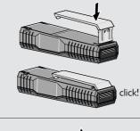
To ensure a reliable use, do not use zinccarbon batteries. Change batteries when battery sym-
